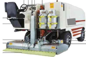
A: Snow tank B: Board brush C: Water tank D: Wash water tank E: Driver seat F: Conditioner
